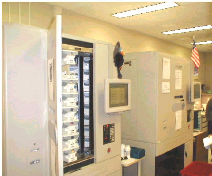
*The robots are metal cabinets, approximately six feet high, five feet wide and four feet deep. There are 520 cells which each hold between 100 and several thousand pills. Based on a computer program and a database of prescriptions, the robot will rotate the cells until the appropriate individual pills are above the dispenser and dropped into plastic bags. The bags are sealed, and the inmates' names and time of dispensation are entered.*
