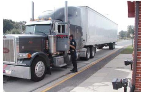
5. Vehicles in violation are directed to a large lot. This area is also used to perform safety inspections. On the left is a covered “pit” which allows inspectors to walk underneath vehicles as they perform such inspections.
